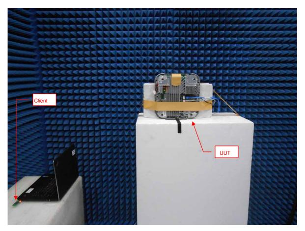
Note: Stating WiFi Module was installed in test fixture with heat sink for the test.
