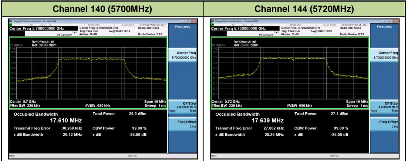
**802.11ac-VHT40 26dB Bandwidth & 99% Bandwidth - Ant 1**
