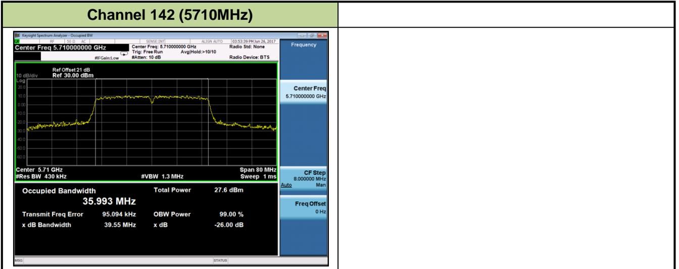
**802.11ac-VHT20 26dB Bandwidth & 99% Bandwidth - Ant 1**
