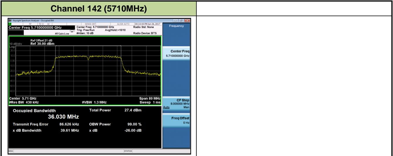
**802.11ac-VHT80 26dB Bandwidth & 99% Bandwidth - Ant 1**
