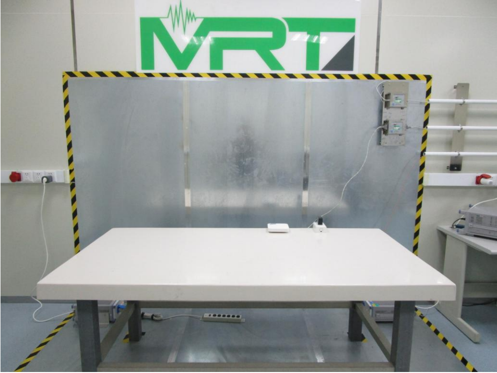
Description: Back view of Conducted Emission Test Setup (Test Mode 1)
