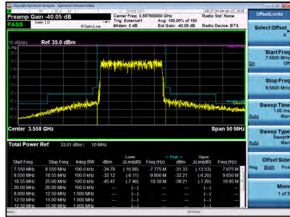
OBW 1 Carrier 15MHz 256QAM 3557.5 MHz
