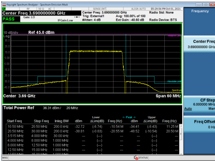
Test Model 3.1a, Modulation 256QAM, Channel Frequency 3690 MHz, TX12
