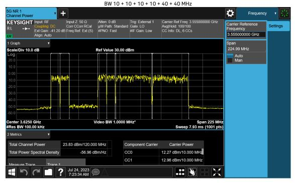
Test Model 3.2 Modulation QPSK / 16QAM Channel Frequency 3555 LTE+ 3565 LTE + 3579 NR +3600 NR + 3630 NR + 3675 NR MHz
