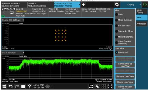
Modulation 64QAM TM3.1 Channel Frequency 3649.995MHz
