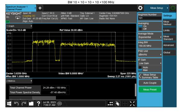
Test Model 3.1 Modulation 64QAM Channel Frequency 3570 NR + 3640 LTE + 3660 LTE + 3680 LTE + 3695 LTE MHz
