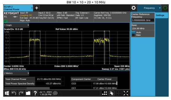
Test Model 3.1 Modulation 64QAM Channel Frequency 3560 LTE+ 3605.01 NR + 3645 NR + 3679.995 NR MHz
