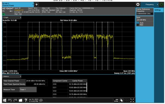
Test Model 3.1a Modulation 256QAM
