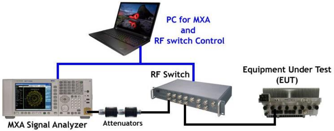
Test Setup for all Antenna Port Measurements
