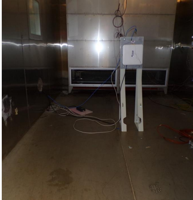
Radio in thermal chamber
