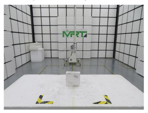
Description: Transmitter Spurious Emissions Test Setup for above 1GHz Internal Antenna
