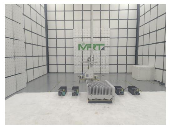
Description: Radiated Spurious Emission Test Setup for 1GHz to 18GHz
