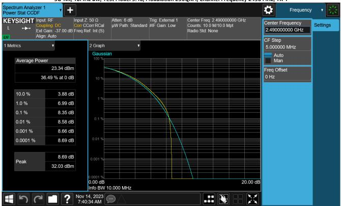
5G-NR, 10MHz BW, Test Model 3.1a, Modulation 256QAM, Channel Frequency 2490 MHz, TX 1
