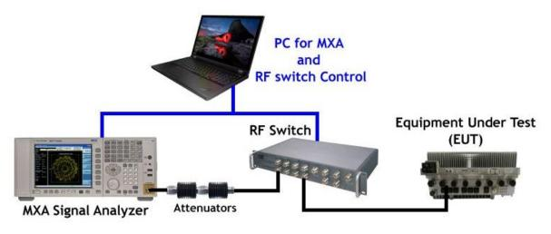
Test Setup for all Antenna Port Measurements
