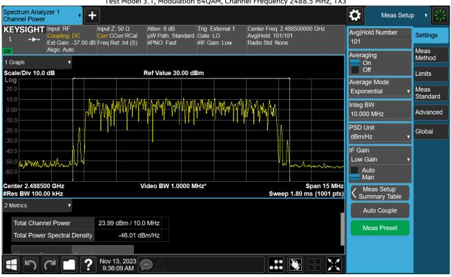
5G-NR, 10MHz BW Test Model 3.1, Modulation 64QAM, Channel Frequency 2488.5 MHz, TX3
