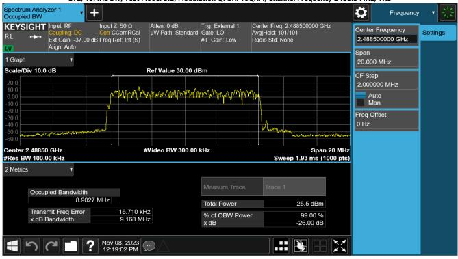
LTE, 10MHz BW, Test Model 3.2, Modulation QPSK/16QAM, Channel Frequency 2488.5 MHz, TX3
