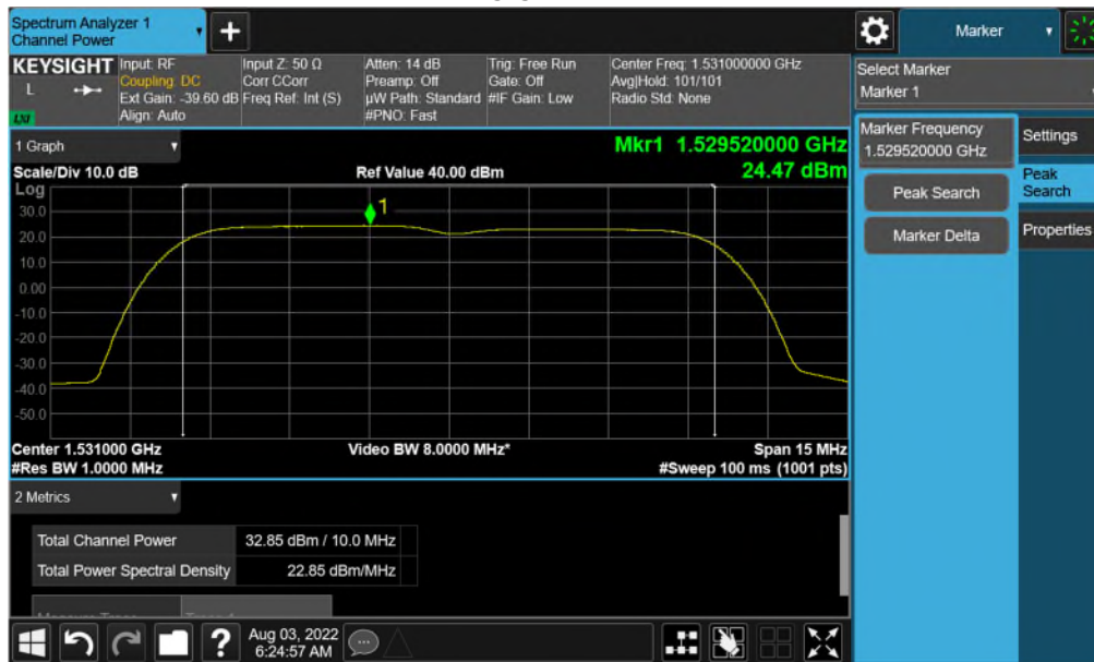
PSD – 2C 5G-NR+LTE 33dBm Test Model 3.1a Modulation 256QAM Channel Frequency 1528.5 +1533.5 MHz 5+5 MHz BW
