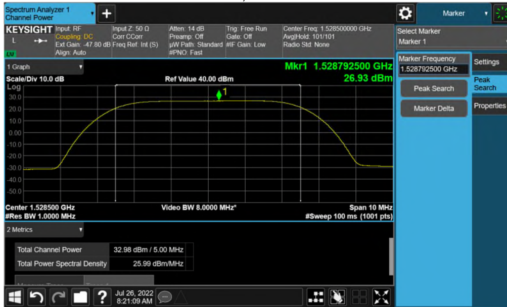
PSD – 1C LTE 33dBm Test Model 3.1 Modulation 64QAM Channel Frequency 1528.5 MHz TX1, 5MHz BW
