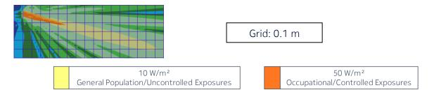
Figure 9 - Side view of the power density for the time-averaged actual maximum transmitted power of 0.7 W and the beam oriented in azimuth =  $0^{\circ}$  & elevation =  $+15^{\circ}$  (EU/ICNIRP, Canada, Australia/NZ and US/related)
