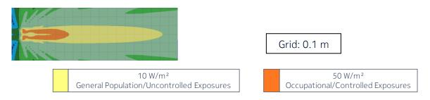
Figure 3 - Top view of the power density for the time-averaged actual maximum transmitted power of 0.7 W and the beam oriented in azimuth = 0° & elevation = 0° (EU/ICNIRP, Canada, Australia/NZ and US/related)
