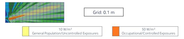
Figure 7 - Side view of the power density for the time-averaged actual maximum transmitted power of 0.7 W and the beam oriented in azimuth = 0° & elevation = -15° (EU/ICNIRP, Canada, Australia/NZ and US/related)
