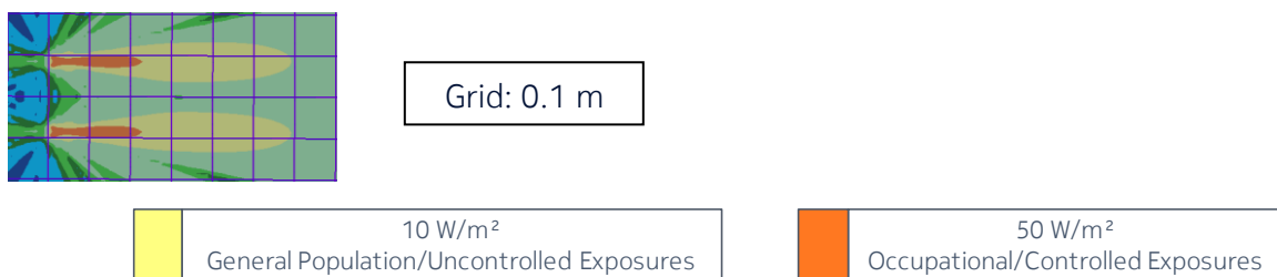
Figure 4 – Top view of the power density for the time-averaged actual maximum transmitted power of 0.36 W and the beam oriented in azimuth = 0° & elevation = 0°
