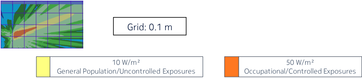
Figure 8 – Side view of the power density for the time-averaged actual maximum transmitted power of 0.36 W and the beam oriented in azimuth = 0° & elevation = -20°
