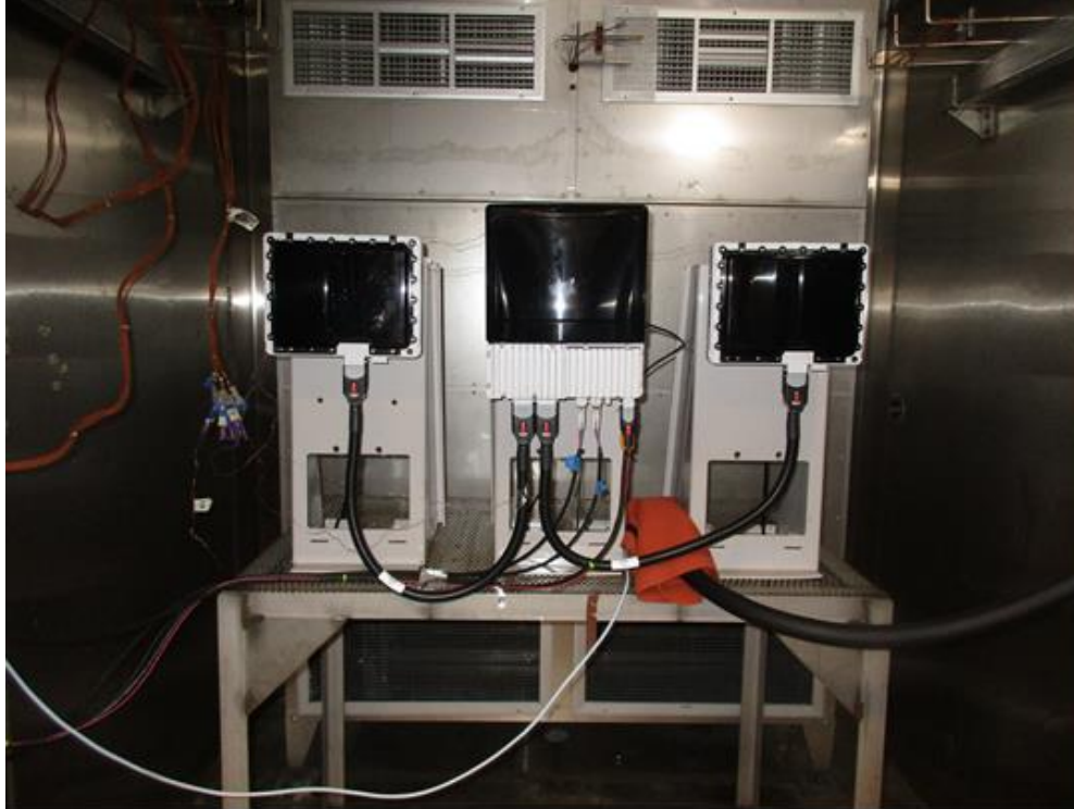
2AD8U24FA3UB in thermal chamber
