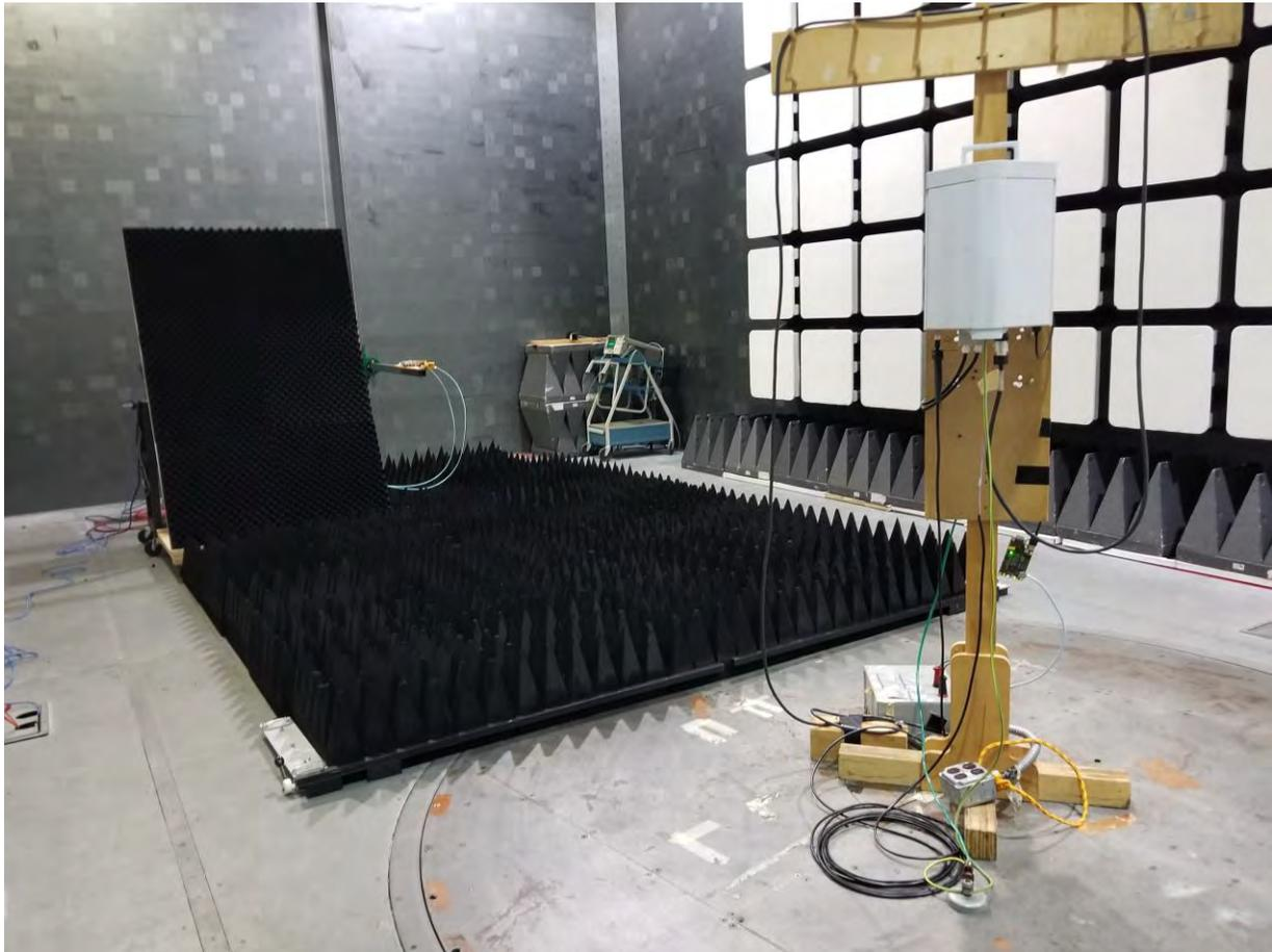
**Radio Measurements 26-31 GHz at 4 m**
