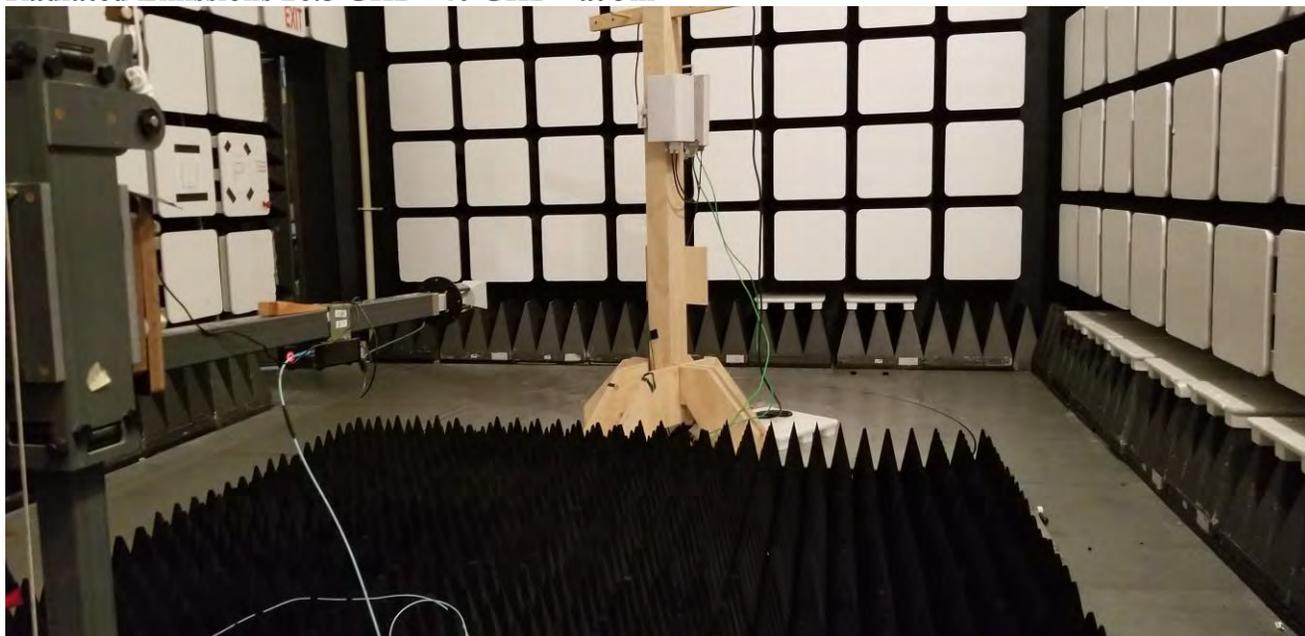
**Radiated Emissions 40 GHz – 60 GHz GHz at 4m**
