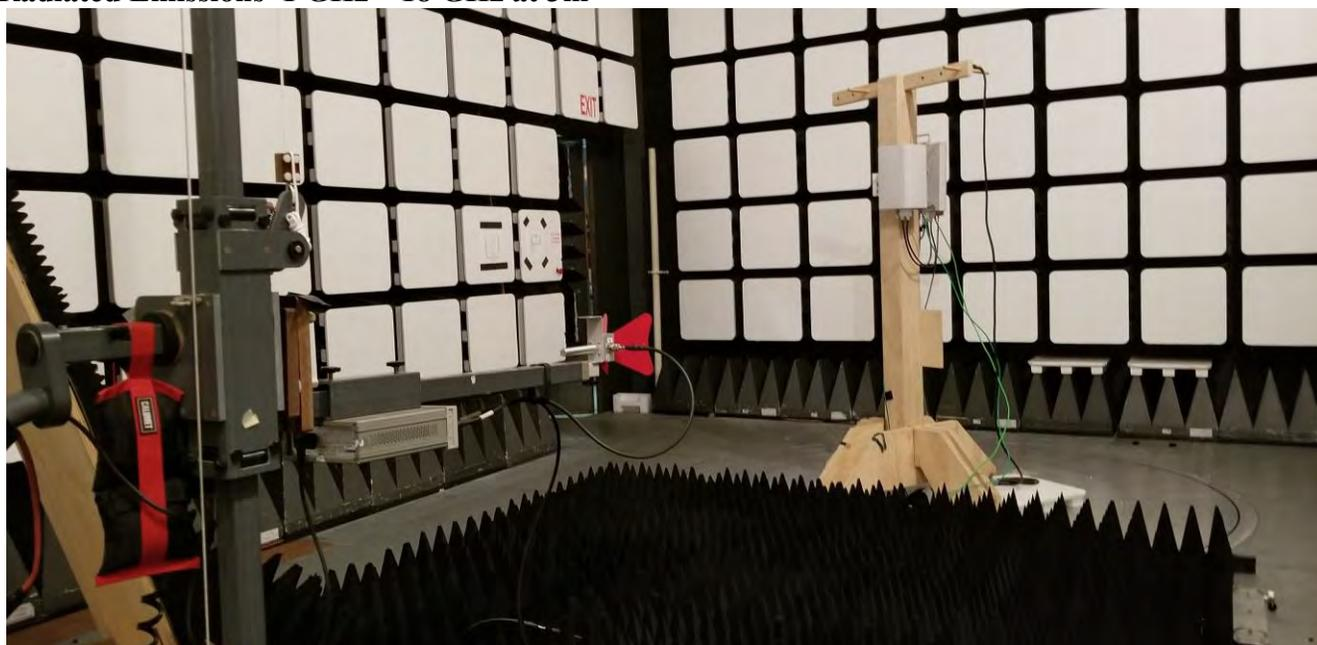
**Radiated Emissions 18 GHz – 26.5 GHz at 3m**
