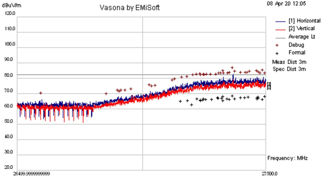
Radiated Emissions Template: Radiated E 1m 26.5GHz-40GHz
