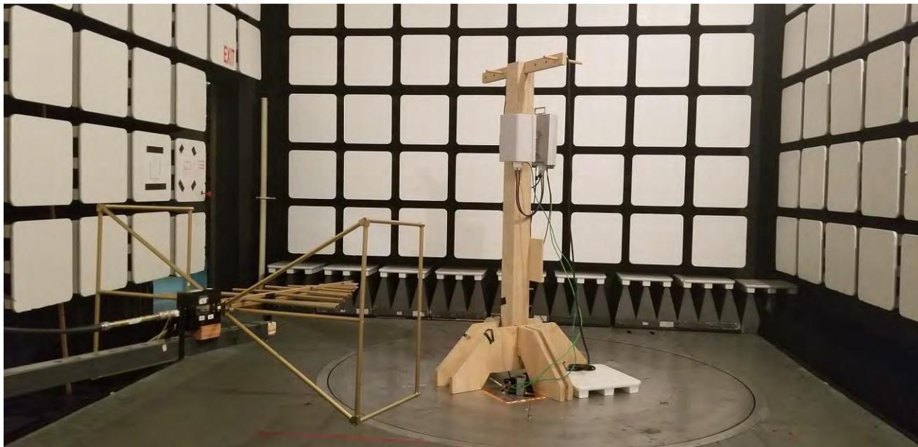
**Radiated Emissions 1 GHz – 18 GHz at 3m**
