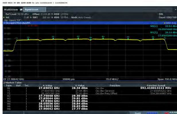
**99% Signal Bandwidth**      **10 MHz RBW, Right, 7 Carrier**
