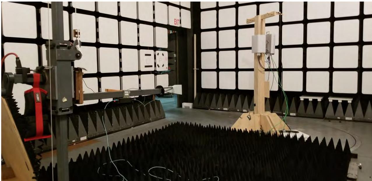
**Radiated Emissions 26.5 GHz – 40 GHz at 3m**
