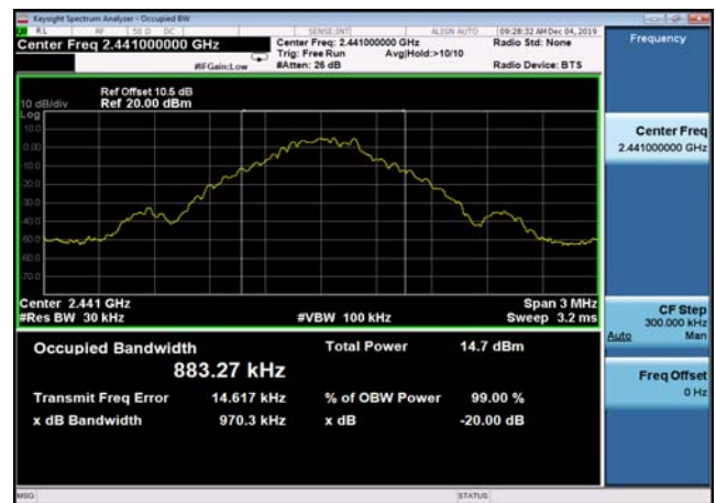
20dB Bandwidth: DQPSK,2402MHz,2DH5
