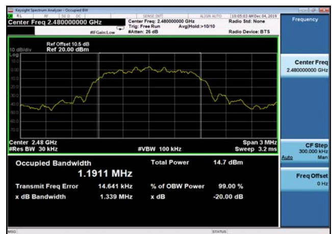
20dB Bandwidth: DQPSK,2480MHz,2DH5
