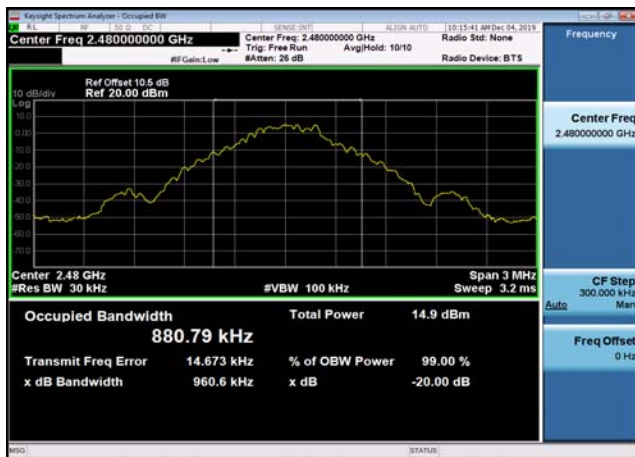
99% Bandwidth: DQPSK,2441MHz,2DH5
