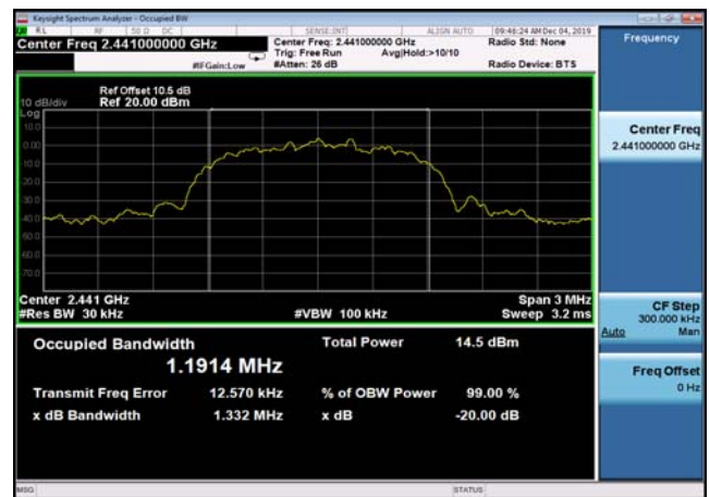
20dB Bandwidth: 8DPSK,2441MHz,3DH5
