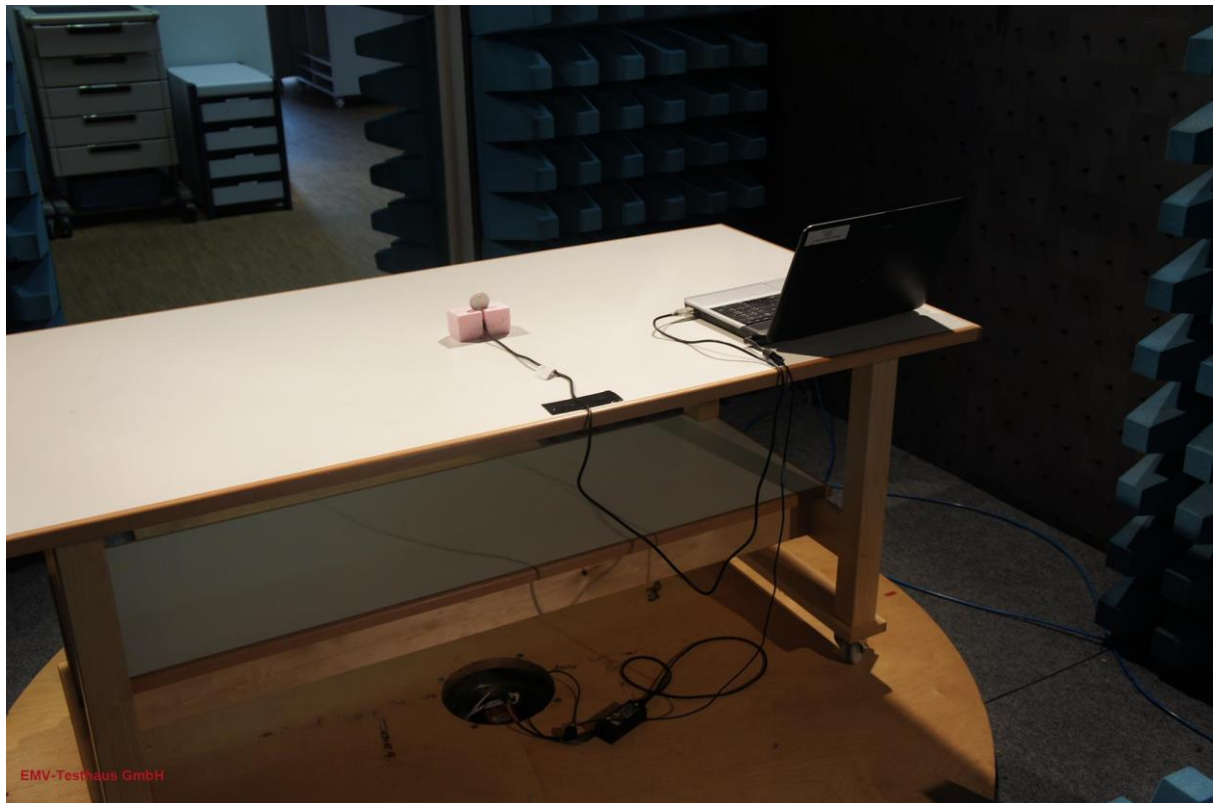
Picture 7: test setup radiated emissions 30 MHz - 1 GHz, CDC, rear view
