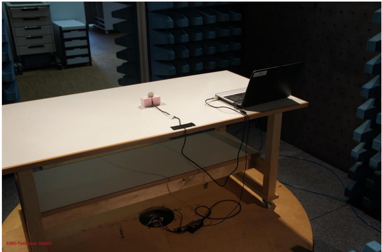
Picture 5: test setup radiated emissions 9 kHz - 30 MHz, CDC, rear view
