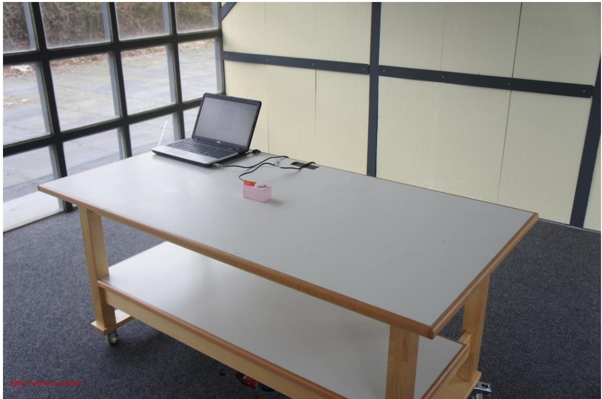
Picture 8: test setup radiated emissions, OATS, front view
