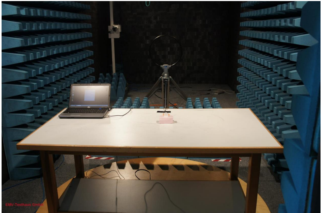
Picture 4: test setup radiated emissions 9 kHz - 30 MHz, CDC, front view
