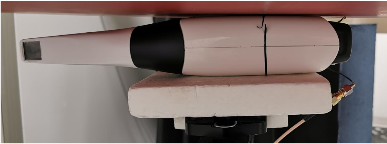
Left side of the DUT against the phantom, 0mm separation distance
