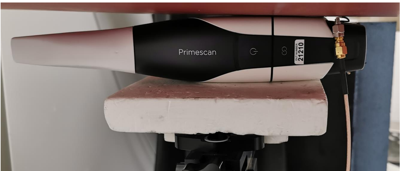
Right side of the DUT against the phantom, 0mm separation distance
