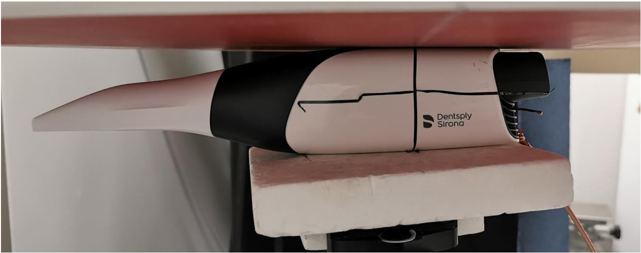
Top side of the DUT against the phantom, 0mm separation distance
