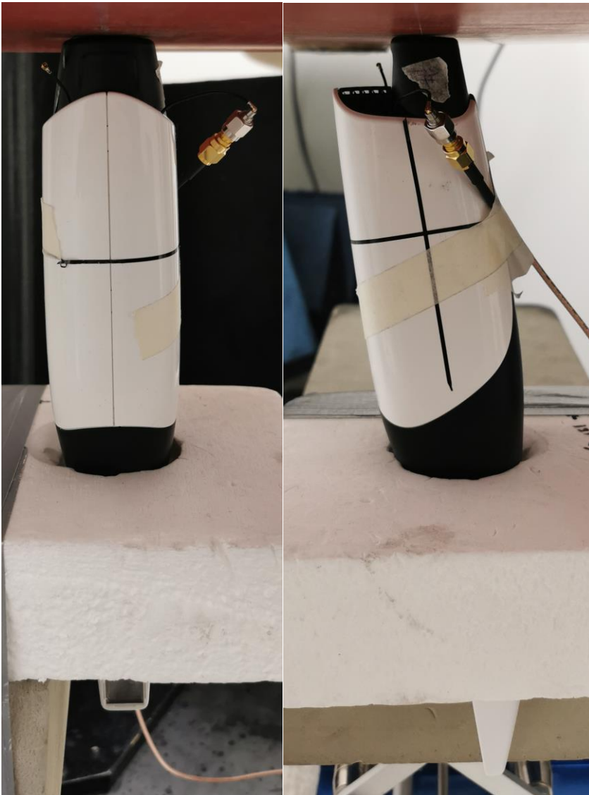
Back side of the DUT against the phantom, 0mm separation distance
