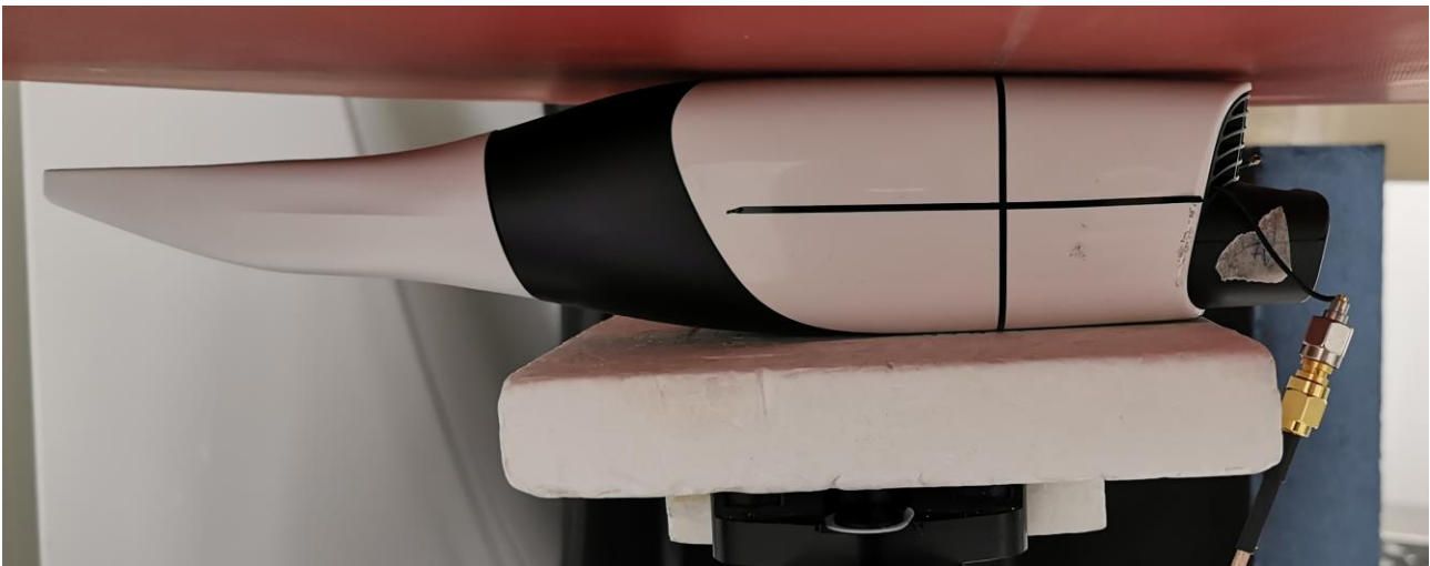
Bottom side of the DUT against the phantom, 0mm separation distance
