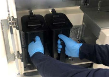
2. Now remove the perforated plate. To do this, press down the central slat and fold down the plate toward the front.
