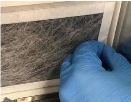
3. The filter has small tabs on the outside. Gently pull the filter forward using the tabs and remove the filter. The used full filter can usually be disposed of in normal household waste.
