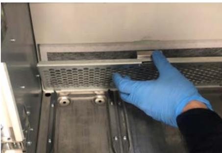
4. Now insert a new activated carbon filter (REF 6745603). Unpack the new filter from the plastic packaging and insert it in the same place. Guide the perforated plate at an angle with the slats first into the groove provided and press the plate until it snaps into place.
