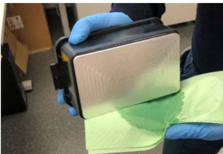
3. First pull the paper towel over the edge and then, if necessary, over the entire surface of the build platform until there is no residual resin left.
