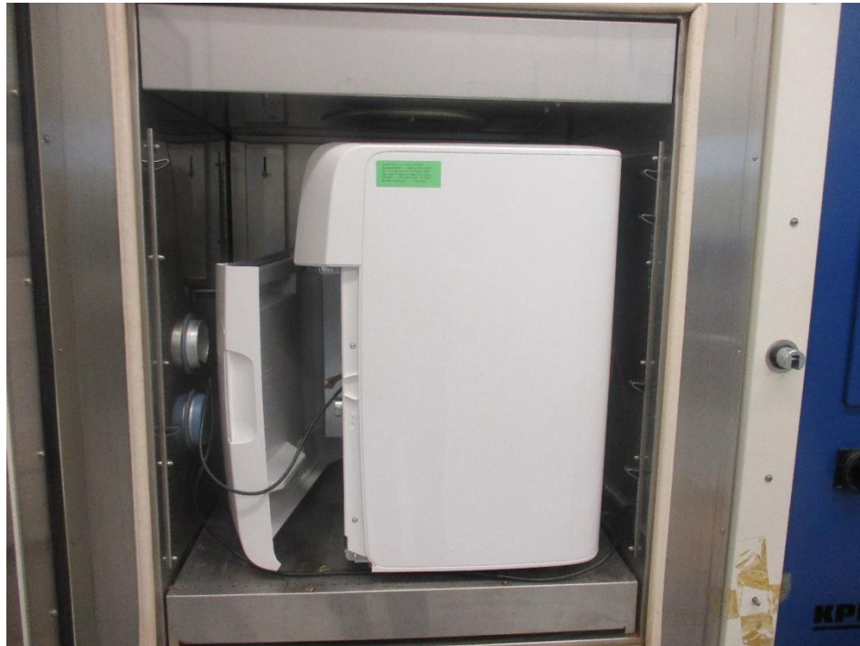
Figure 7 – Test setup for carrier frequency stability
