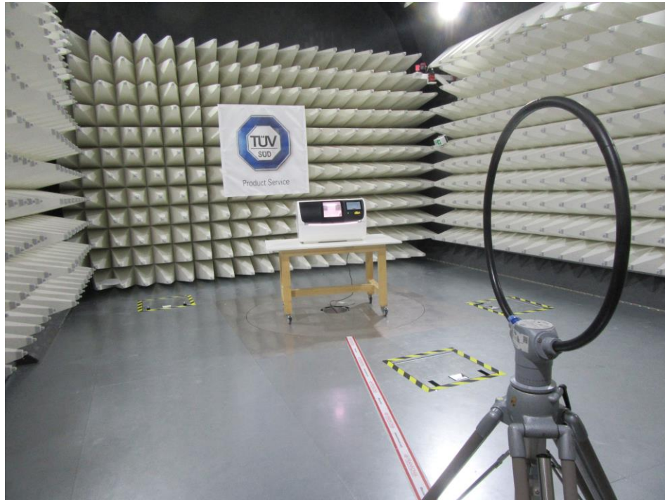
Figure 6 – Test setup for radiated emission 9kHz – 30MHz
