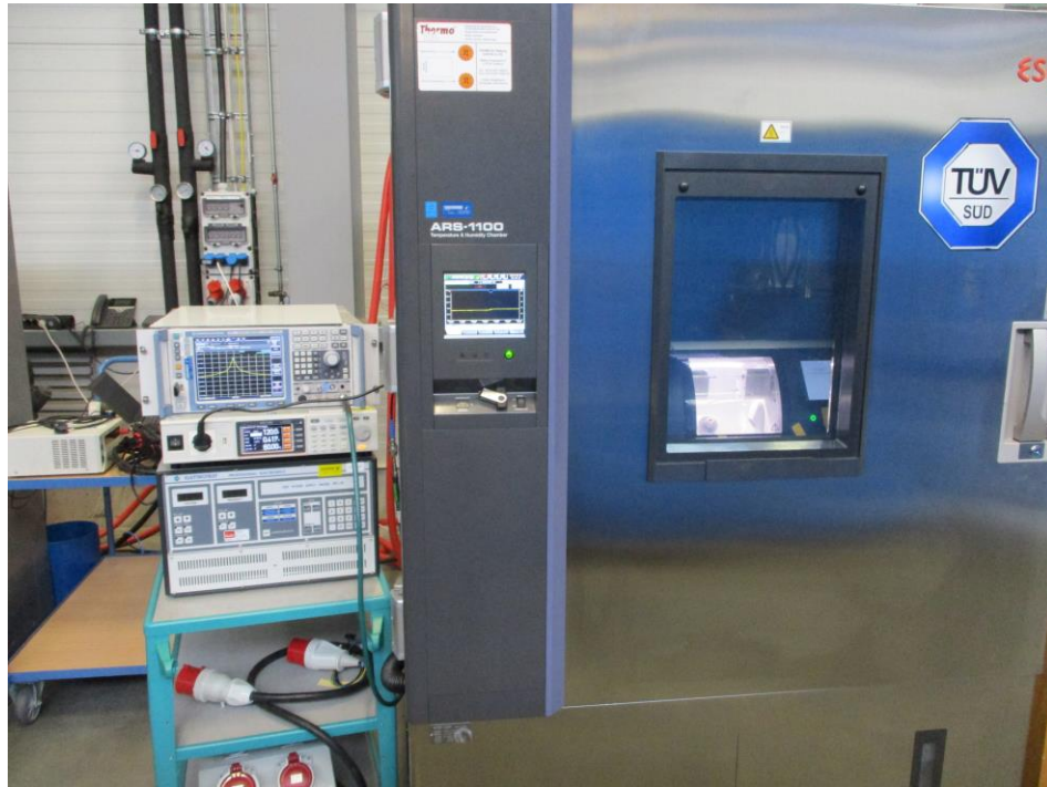
Figure 8 – Test setup for carrier frequency stability
