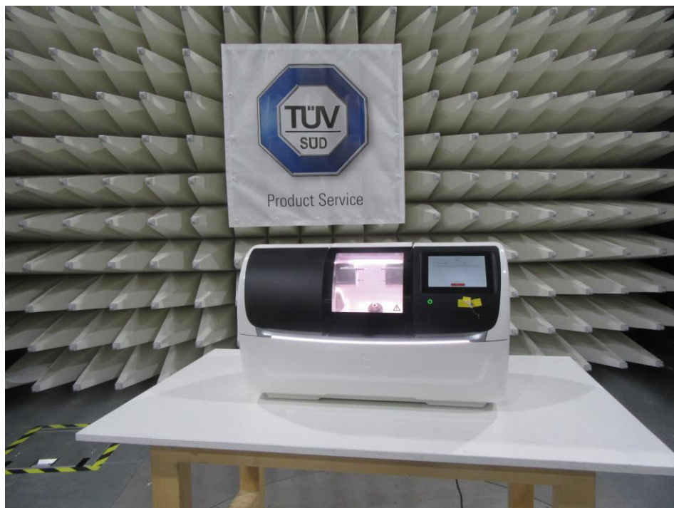
Figure 1 – Test setup for radiated emission 9kHz – 30MHz
