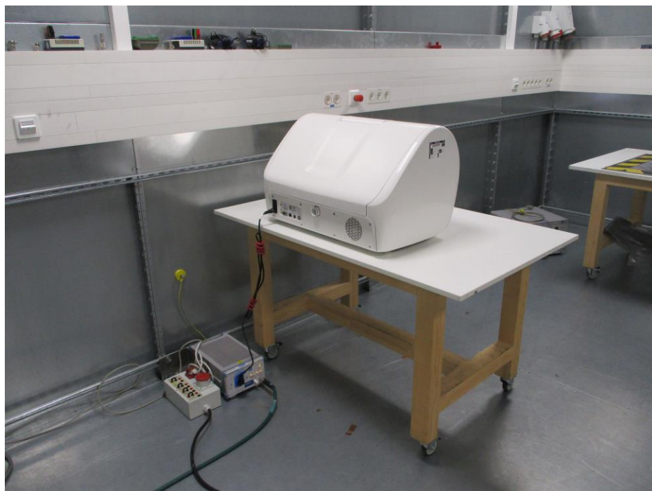
Figure 9 – Test setup for AC Power Line Conducted Emissions
