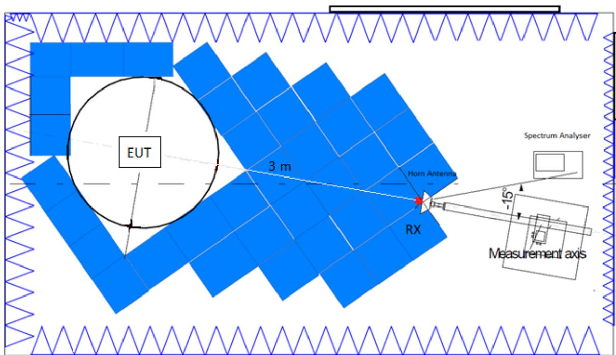
Radiated measurements setup for  $f > 17$  GHz:
