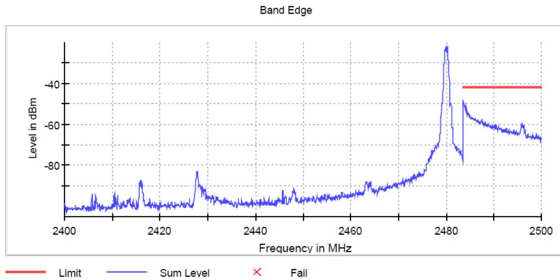
The attenuation of the highest emissions at the band edges is more than 20 dB respect to the highest level of the desired power.
