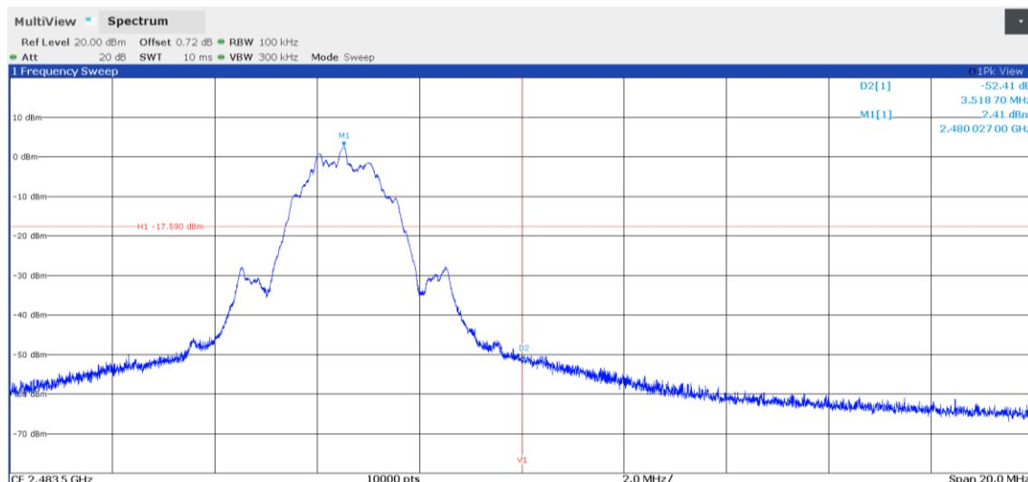
The attenuation of the highest emissions at the band edges is more than 20 dB respect to the highest level of the desired power.
