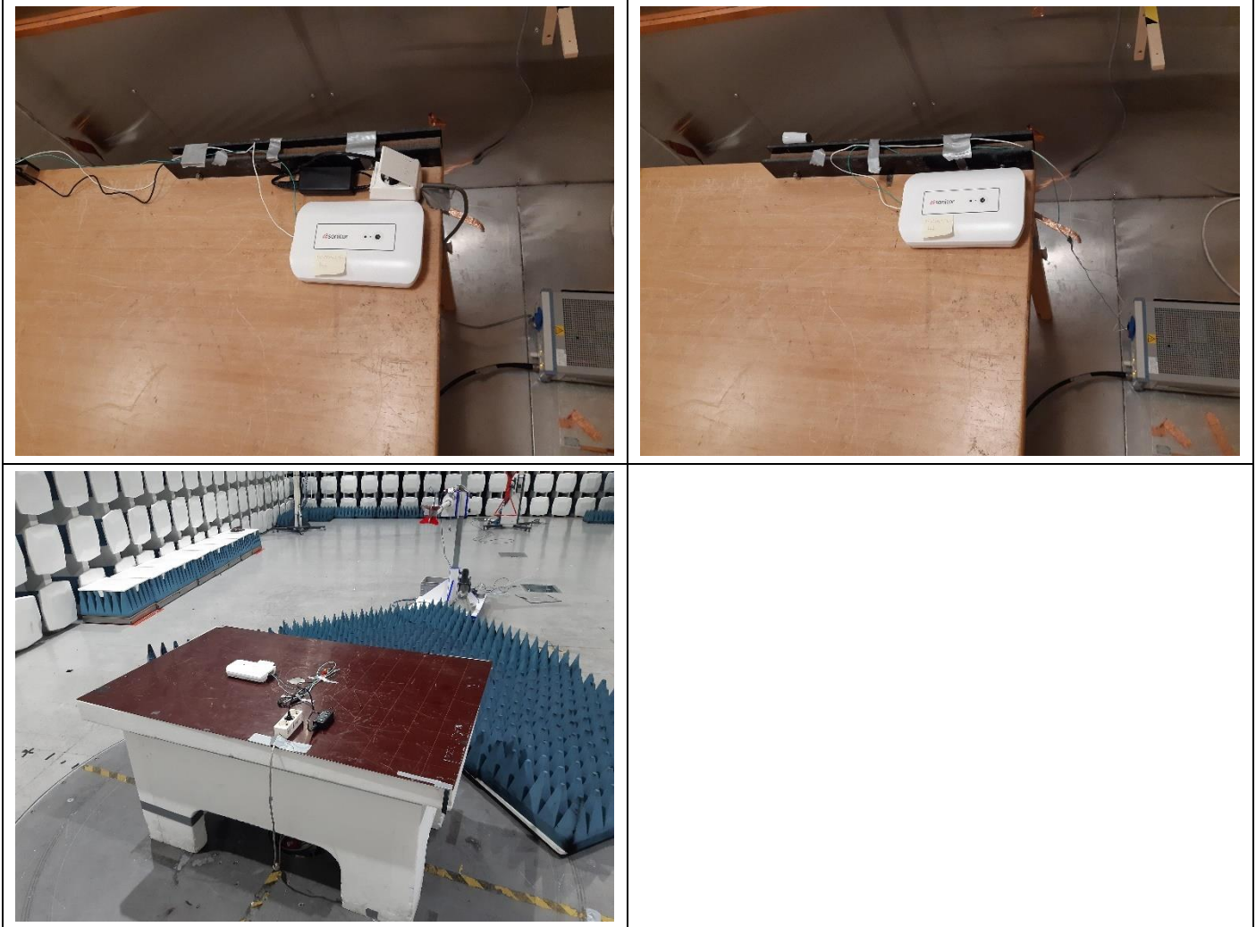
Test set-up for EMC emissions measurements
