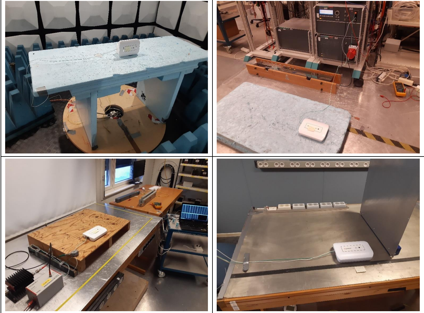
Test set-up for EMC immunity tests
