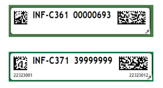
Figure 3: Example of TAB ID label, 57 x 11 mm<sup>2</sup>, with a Datamatrix 2D GIAI to the left and a Datamatrix GS-1 to the right, for INF-C361 and INF-C371.
