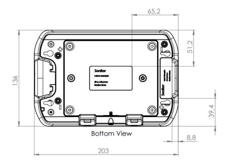
Figure 1: Illustration of label placements (all dimensions in mm).
