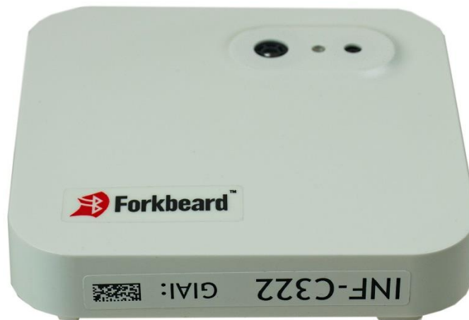
Figure 2 Side view with product number and GIAI label
