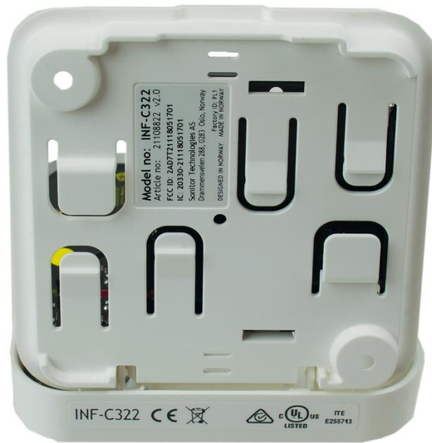
Figure 3 Base view (lid opened) with FCC ID and IC presented on the product label and additional approval marks on the side
