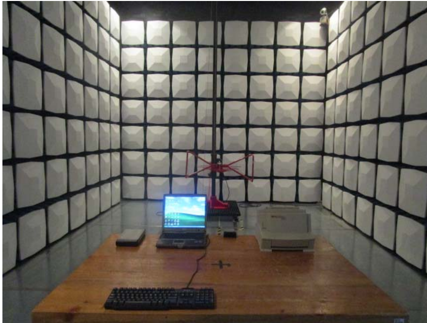
Radiated Emission Below 1GHz –Rear View
