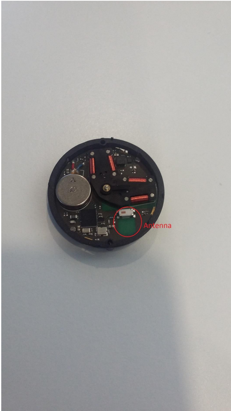
Photo 5: PCB front side view with antenna
