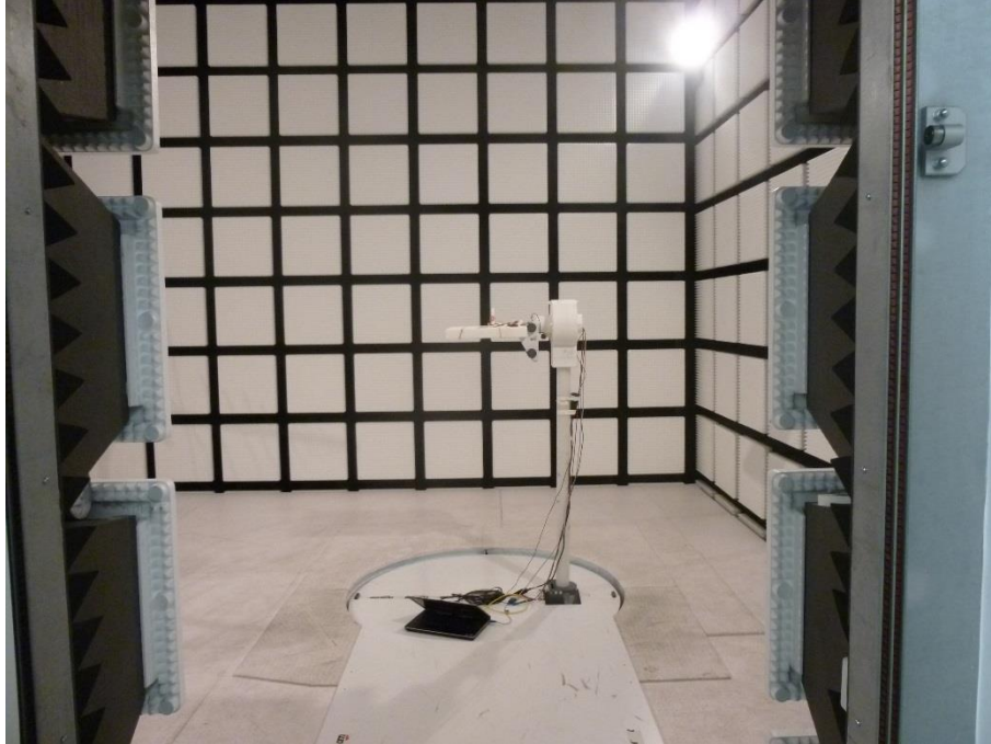
Photo 1: EUT at the anechoic chamber
