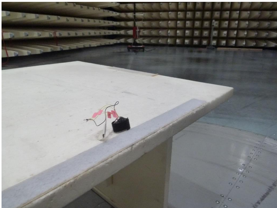
Photo 8: EUT at the semi-anechoic chamber
