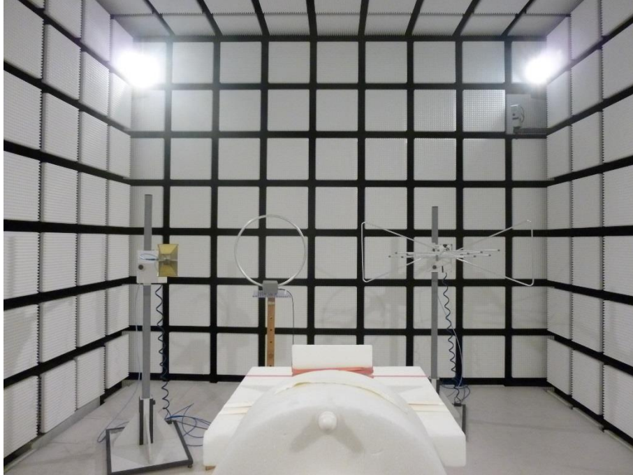
Photo 5: EUT at the anechoic chamber
