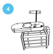
Use holding hook to suspend the light fixture, and free up both hands for wiring.
