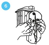
Holding the light fixture with both hands, align the two fixture long screws into the light fixture screw-posts.
