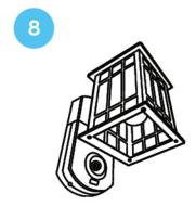
Adjust the angle of the camera lens loosening up the locking ring. Use 2 fingers and turn it counter clockwise. Lock up it back up by turning the locking ring clockwise. For final adjustment, see the video feed on the phone after WiFi setup.
