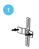
Insert fixture long screws and nuts into the Bracket as shown.
