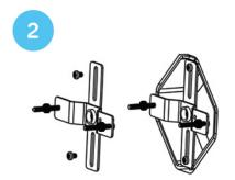
Fasten bracket to junction box with the shorter screws.
