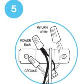
Use wire nuts to connect: Black to Black wires. Insert both wires all the way into the nut and twist until secure. Then repeat for the white wires and for the ground wires.
