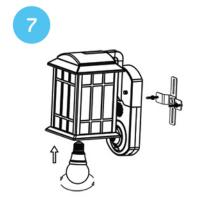
Mount the light fixture to the long screws as shown, then install both decorative nuts. Install a light bulb and apply silicone sealant between wall and light fixture (optional).
