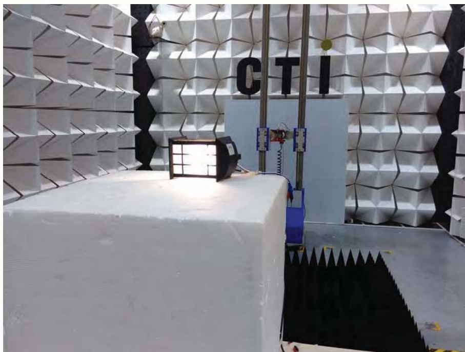
Radiated spurious emission Test Setup-2 (Above 1GHz)
