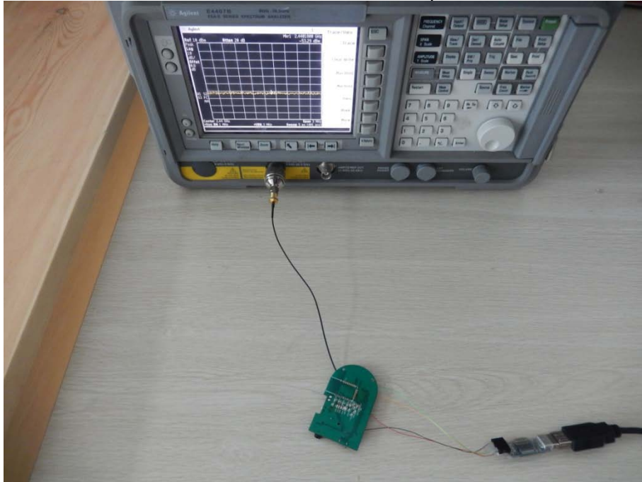
DSS&DTS RF conduction test photos
