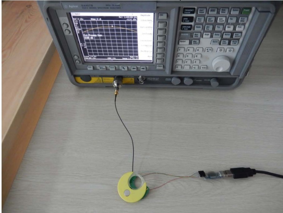
DTS RF conduction test photos
