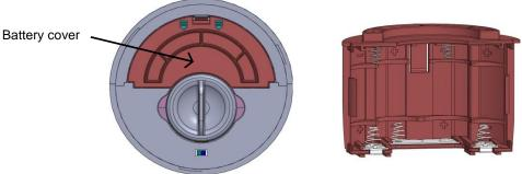
Put the battery cover back then close the bedplate by turning it to the left
