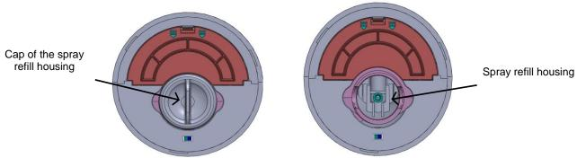
Screw by hand the cap of the spray refill housing then close the bedplate by turning it to the left
