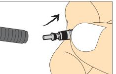
3. Screw the Tire Pressure Sensors into the Presta stem. Use the wrench tool to tighten it securely.
