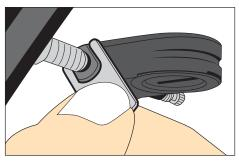
4. Adjust the Sensor to align with the wheel
