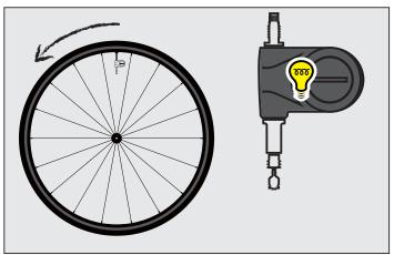
Push the wheels and activate the Sensor. The indicator light will turn on.
