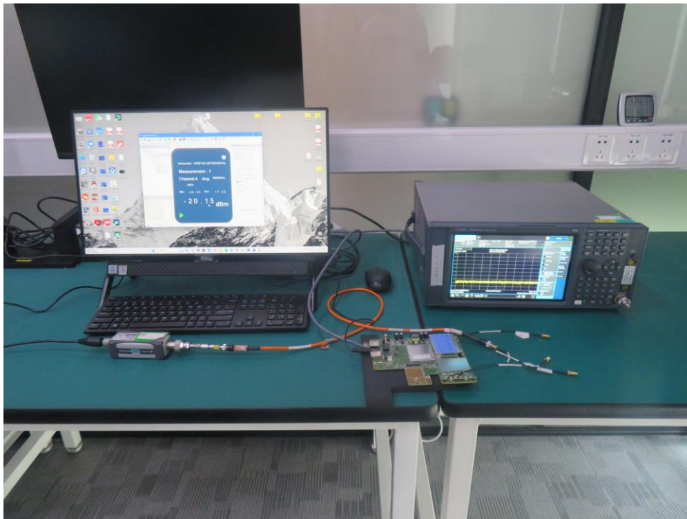
Description: Conducted Test Setup
