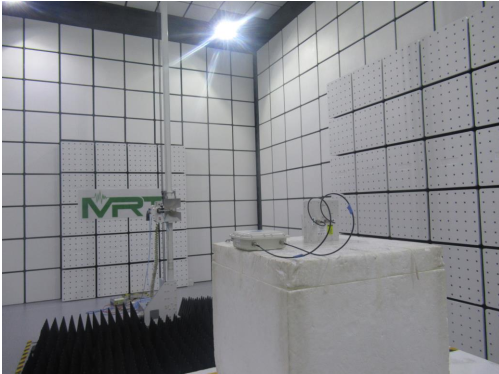
Description: Radiated Spurious Emission Test Setup for Above 18GHz (AX52)
