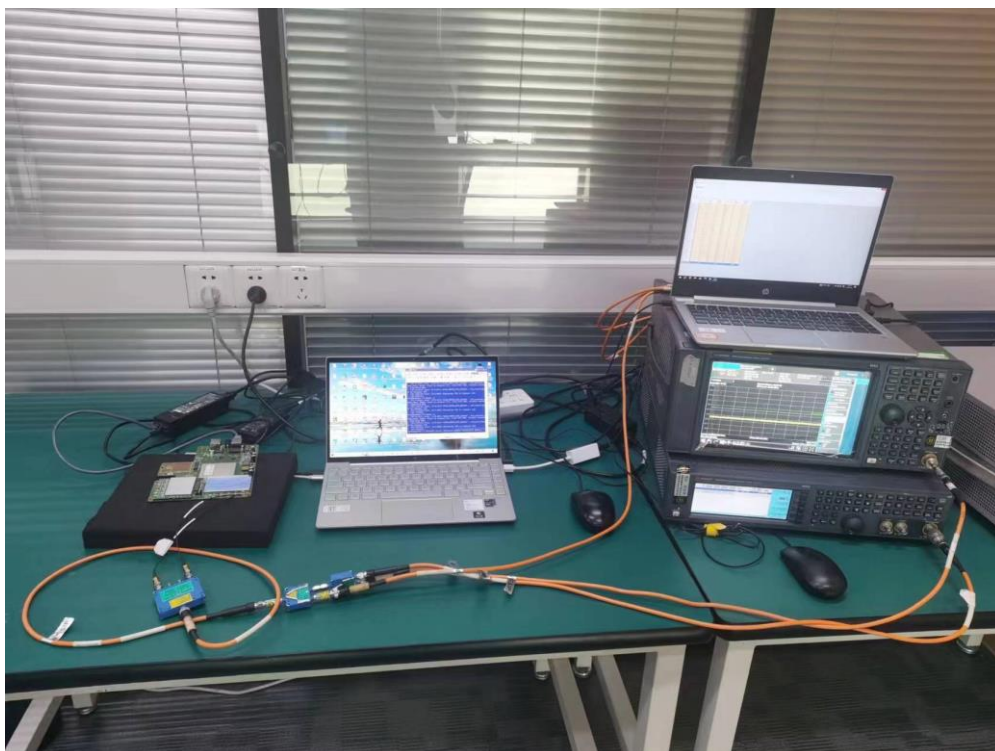
Description: DFS Test Setup(Master Mode)
