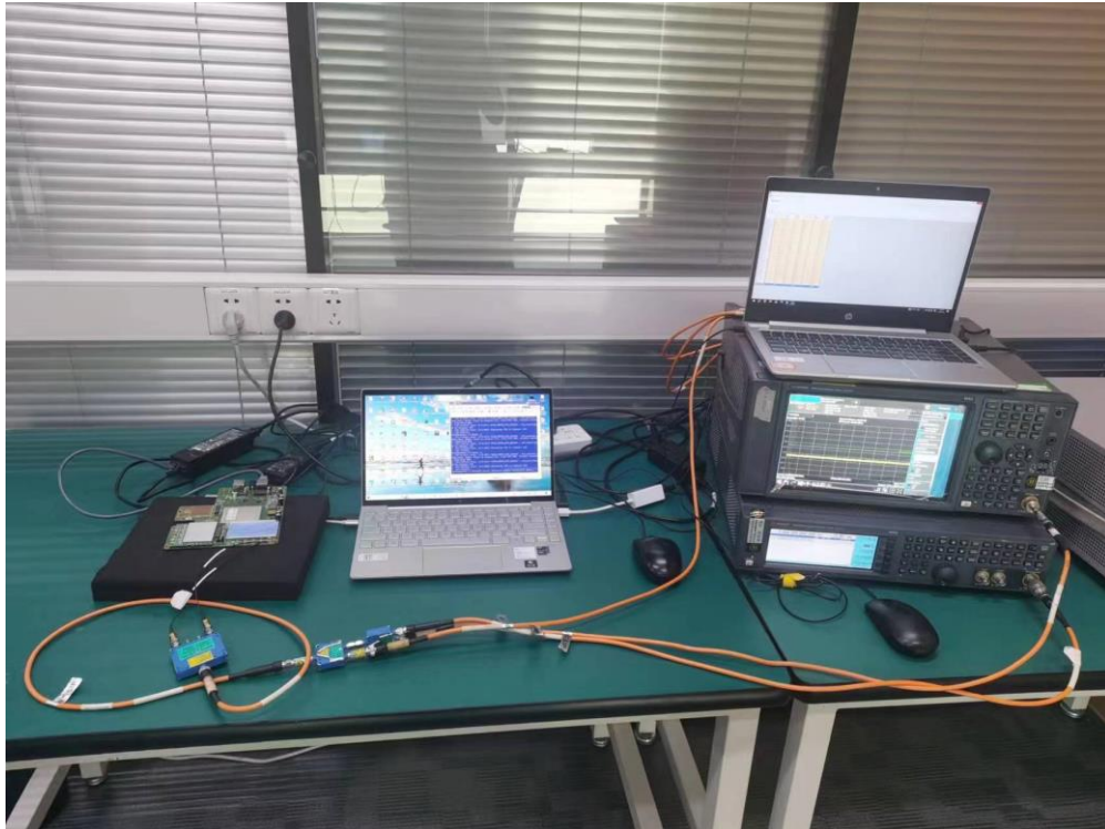
Description: Dynamic Frequency Selection Test Setup(Client Without Radar Detection)
