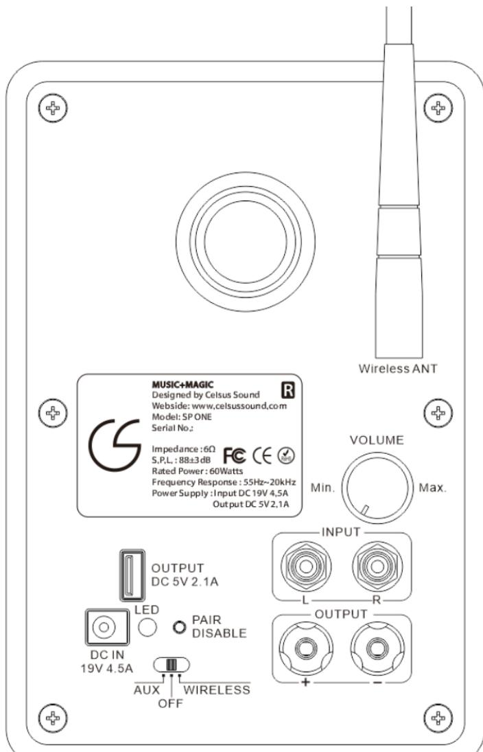
The 5V charger output on the back of SP-One can be used to power an external WiFi Audio receiver or use as a charger for your mobile device.
