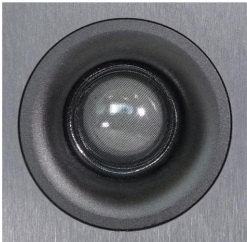
The soft-dome tweeter's high-energy magnetic flux and self-cooling capability together produce an audibly clearer signal.
