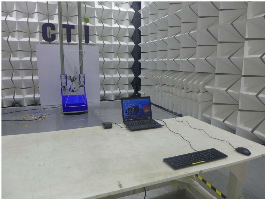
Radiated emission Test Setup-2 (30MHz-1GHz)
