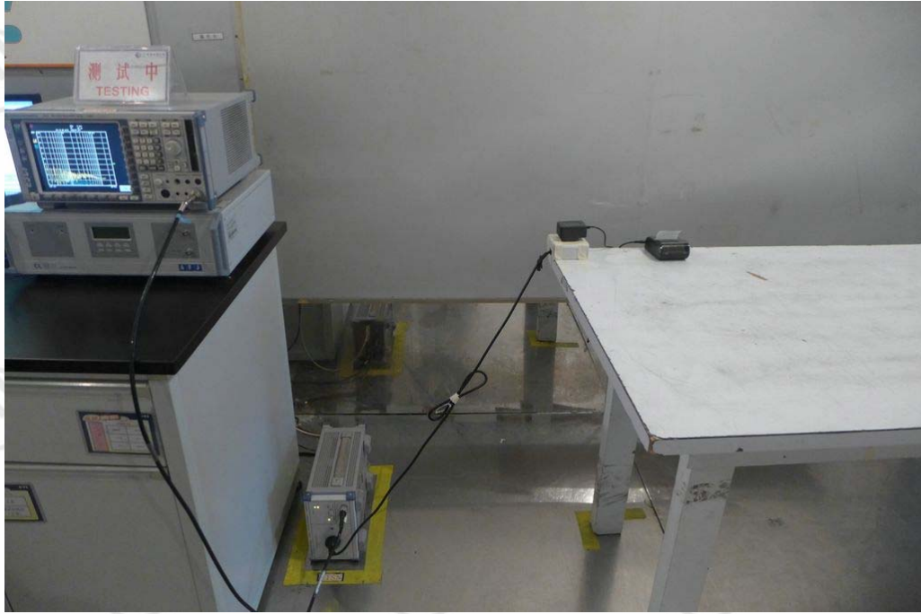
Conducted Emissions Test Setup
