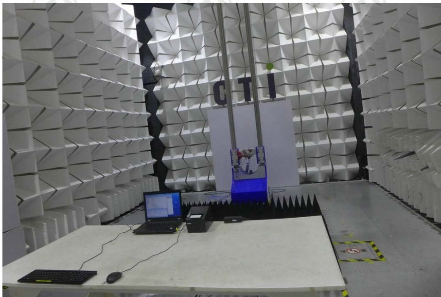
Radiated spurious emission Test Setup-3(Above 1GHz)
