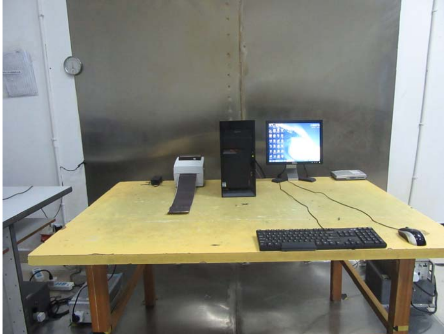
Conducted Emissions – Front View
