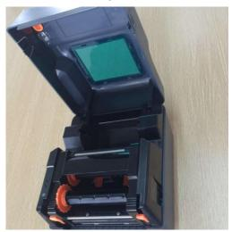
3. Make the left side of recovery shaft (Hexagonal side) pressed into the ribbon recovery wheel, and then assembles the right side
