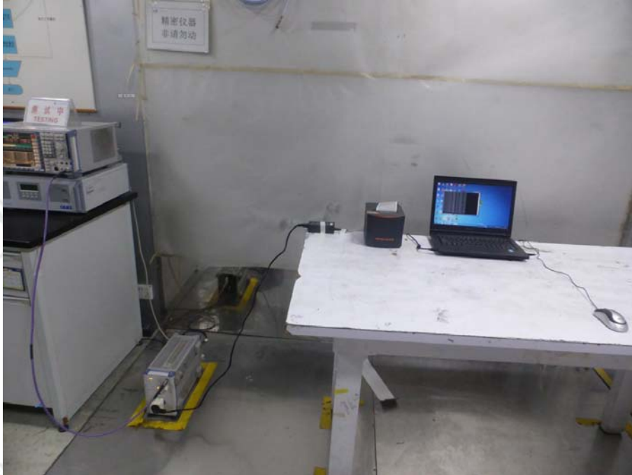
CONDUCTED EMISSION TEST SETUP
