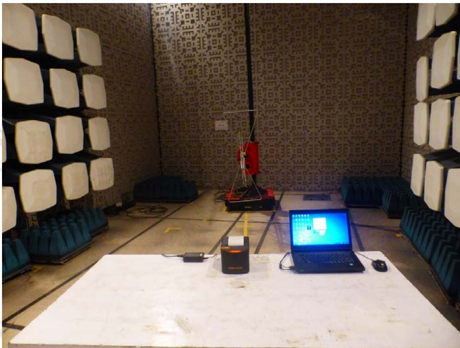
RADIATED EMISSION TEST SETUP
