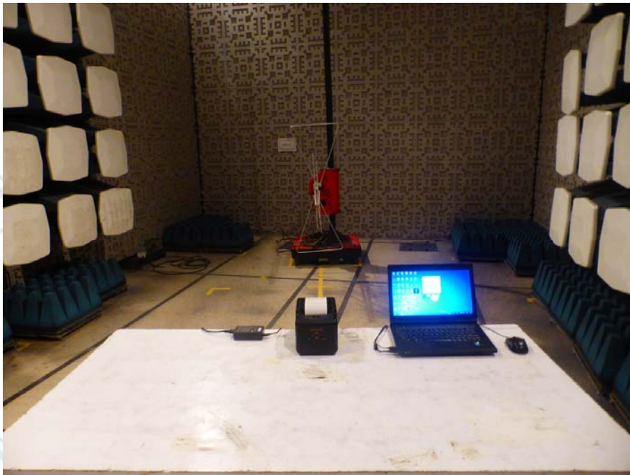
RADIATED EMISSION TEST SETUP
