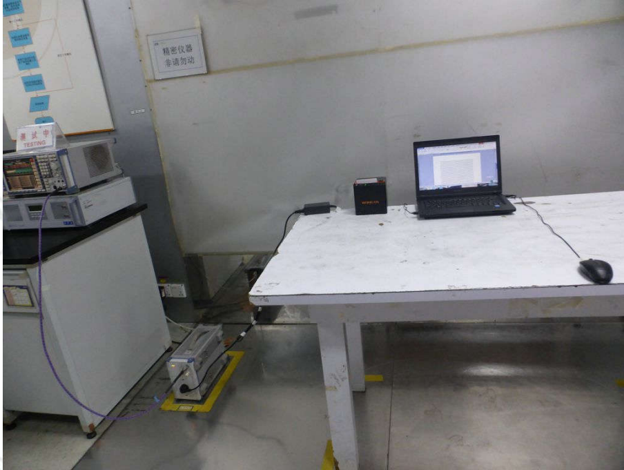
CONDUCTED EMISSION TEST SETUP
