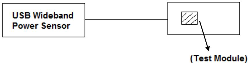
The EUT (Equipment under the test) which is coupled to the USB Wideband Power Sensor; the RF load attached to the EUT antenna terminal is 50Ohm; the path loss as the factor is calibrated to correct the reading, all test result in power meter.
