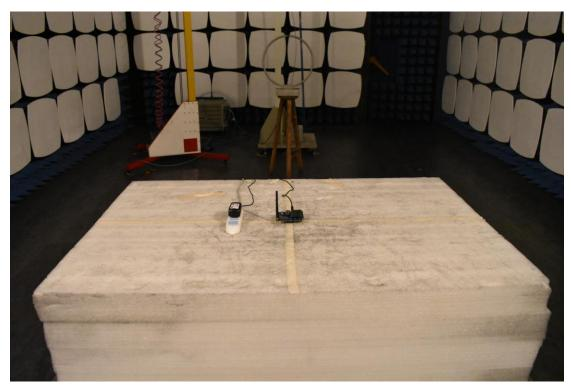
3. Radiated emission (9KHz-30MHz)
