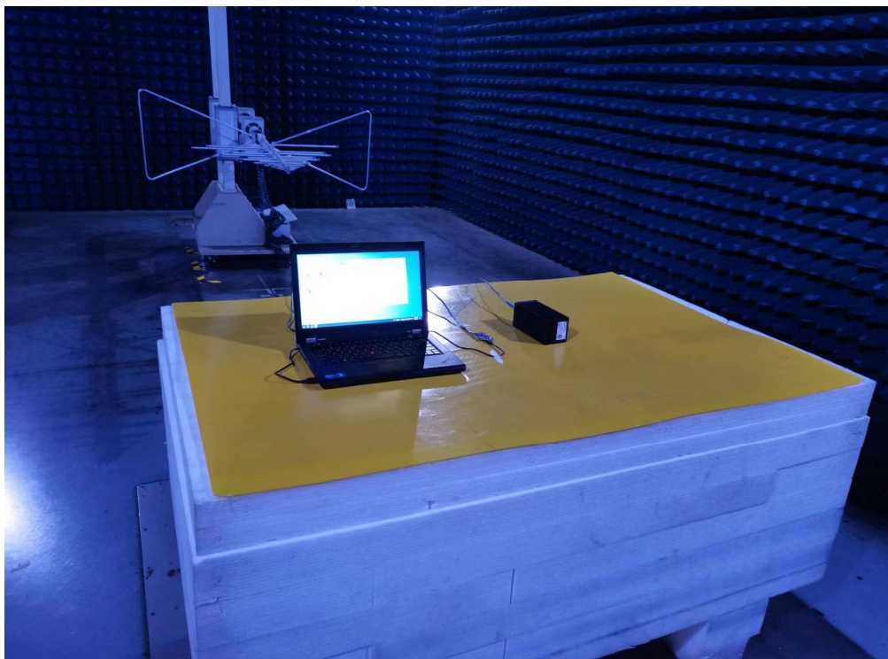
Photo of Radiated Emission Measurement (Above 1G)
